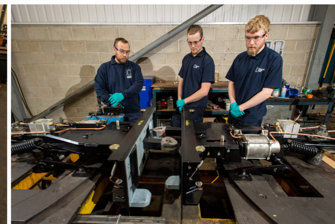
Apprentices Thomas Roberts (centre) and Brendon Dunbar (right) with a wedgelock coupler
