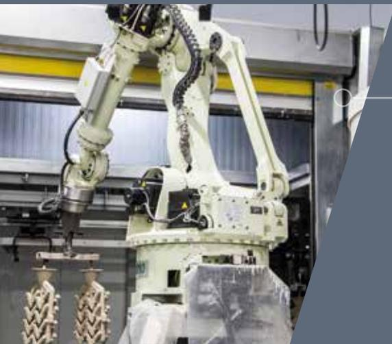
3. PMMA pattern coated by robots to create mould.
