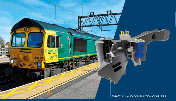
William Cook Rail designs, manufactures and overhauls tightlock couplers for passenger and freight trains. This proven and robust design can be adapted to different types of rolling stock, and supplied with a pneumatic coupling and uncoupling system.
