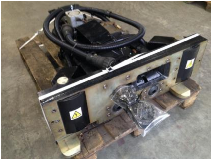
Repaired Intermediate Wedgelock Coupler with contact boxes and TBTC Boxes (Northern Line)
